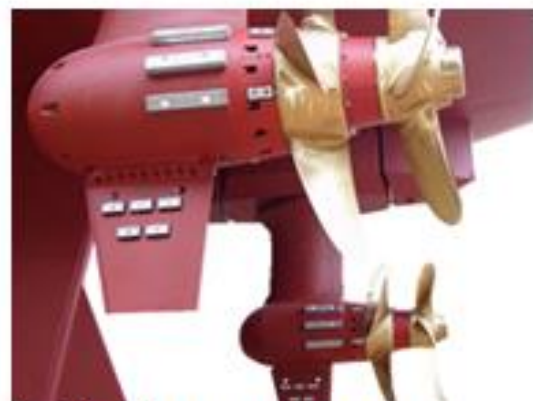
Electric propulsion system
