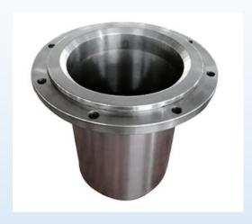
Shaft couplings supplied with shafting, coupling tapers are bedded to shafts at the factory to achieve a fit, of 70% minimum. The fit of keys and keyways will also be inspected. When a coupling is supplied on its own, the fit to the shaft will need to be checked on site. The taper of the coupling, or shaft, should be scraped to produce a fit of 70% minimum. The key should be inspected for a correct fit in both coupling and shaft.
