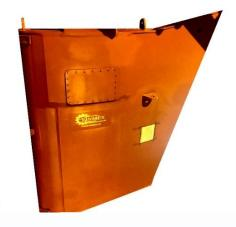
The balance rudder blade is usually a rudder of which the axis this between the front and back of the rudder blade. it acts as a balance when steeing.
